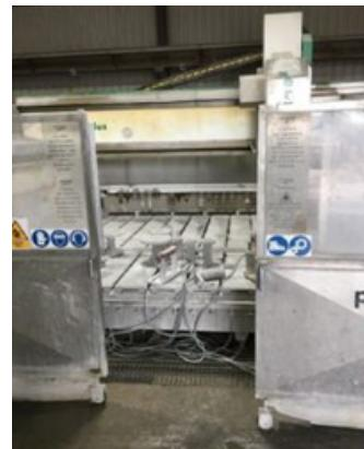
There was no interlock guard on the sliding doors meaning they could be opened while the machine was in operation
